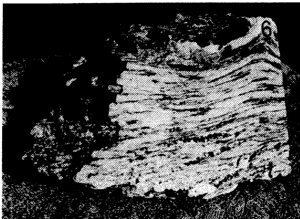
Figure 7. Attenuated layers of dolomite and fractured and rotated dolomite fragments are visible in this sample. The behavior of the dolomite is more brittle than that of the gypsum. Size of sample is 14 cm × 10 cm. NUMBER ON SAMPLE DOES NOT REFER TO FIGURE NUMBER.
